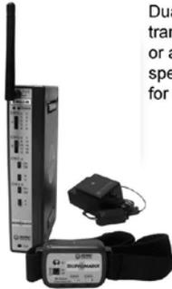
Dual-channel BioNomadix pairs include a wireless transmitter and receiver for either two of the same signal or a combination of signals. BioNomadix are optimized for specific signal types and provide high quality data suitable for advanced analysis, such as heart rate variability.
